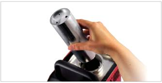
The optimum thermal coupling from the block to test item is achieved with the correct adapter sleeve. Ideally, the internal diameter of the sleeve is 0.5 mm larger than the outer diameter of the test item. With the aid of the adapter sleeve, straight temperature sensors of virtually any length and diameter can be calibrated. The dry block covers the entire temperature range without the need to change the calibration medium. Viscosity, flash points or outgassing are of no concern.
